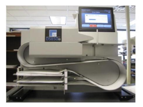
The DS850 accurately records all votes as marked by the voter and is capable of meeting or exceeding the 1.5 million mark test as stated in Volume 1, Section 2.1.1 of the 2005 VVSG. Voter accumulation records are saved on the machine's hard drive and can be transferred from the hard drive to a USB flash drive.
